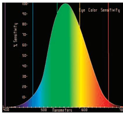
**Figure 1.** The human eye’s sensitivity to color is shown in this illustration. The color vertical lines are the wavelengths of common lasers.
