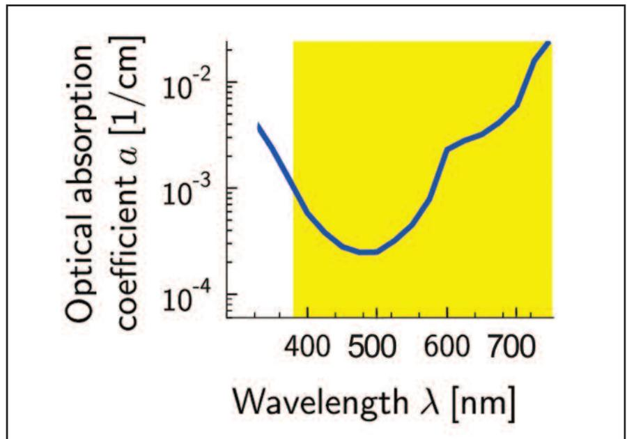
**Figure 2.** The optical absorption of light by water in the range visible to humans is least in the wavelengths of blue. (Adapted from Hale and Querry, *Applied Optics*, 1973)
